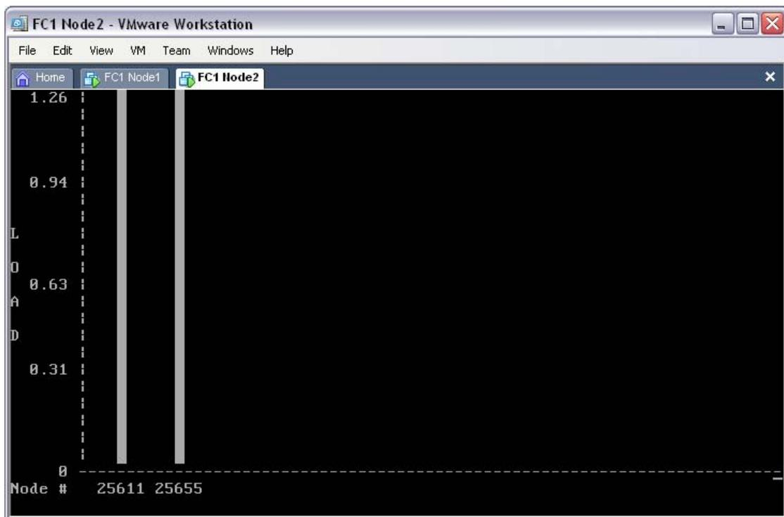
Move to the second node. At the system prompt run the command “mosmon”. You should see an identical load display to the first node.
