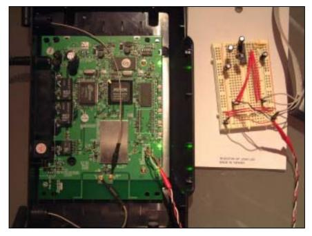
We entered into the final test, uncertain of some of the previous measurements, but unable to prove their accuracy to ourselves. Finally, with the circuit connected, and the Belkin rebooted, output came through perfectly (as readable ASCII).
