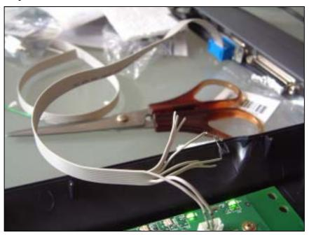
If it hadn't have been for the remarkably well timed output (that appeared to run in sync with a 2-3 second kernel boot sequence) we would have gone back to repairing the TTL to RS232 circuit as a priority. Shown here – the garbage output coming from the Belkin, with a direct connection to the PC serial port;
