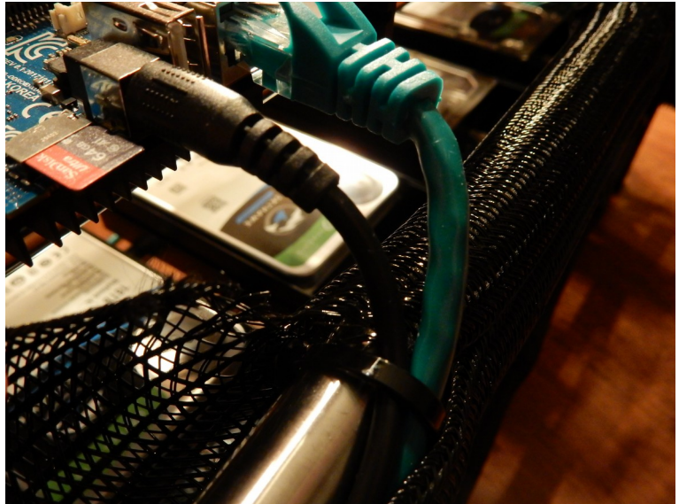
Figure 16: Node cables tightly cable (zip) tied to the front rail
