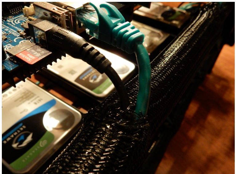
Figure 17: Cable trunk on the top shelf, with closed braided wire wrap
