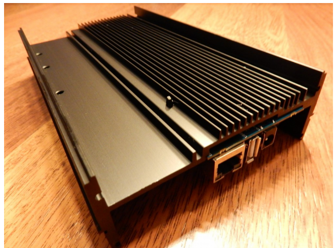
Figure 10: Odroid HC2 – The aluminium enclosure is a heat-sink
